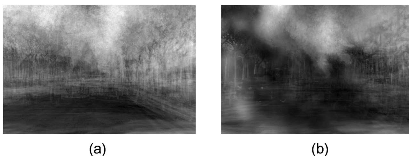
Figure 5. Pixel standard deviation image: (a) Clear image sequence; (b) Dirty image sequence
