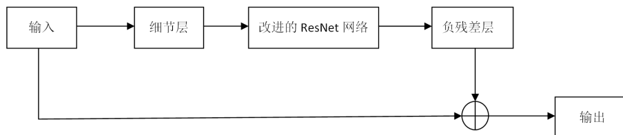
Figure 6. Image derain network structure
