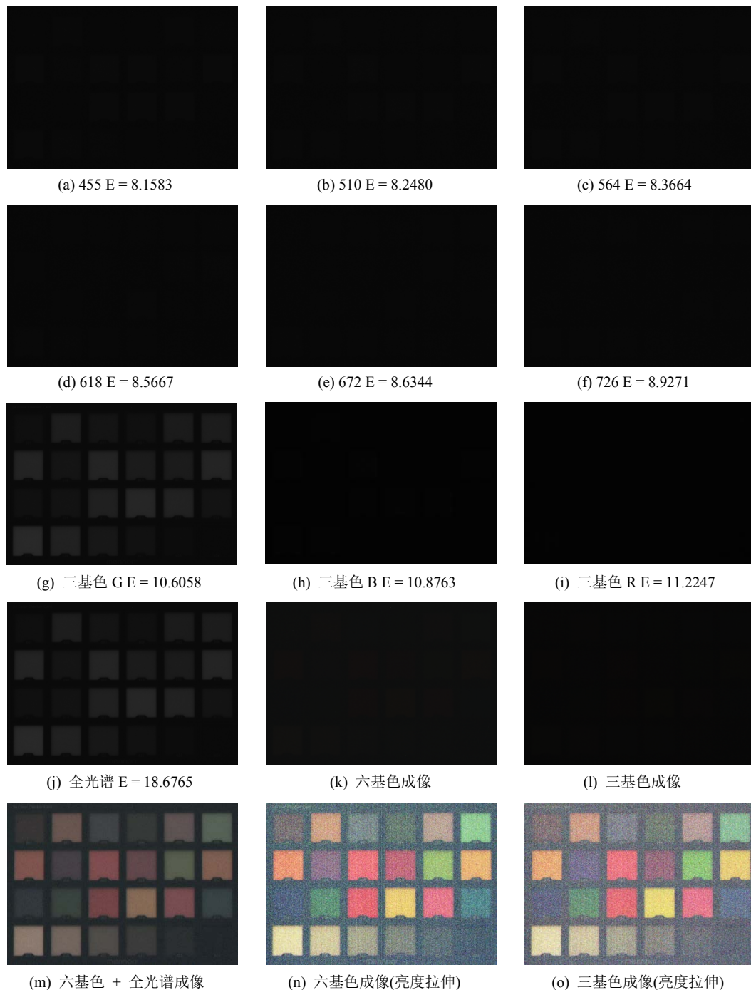
Figure 5. Multi-band image collected by 0.5 lx and color image after fusion 图 5. 0.5 lx 采集的多波段图像及融合后彩色图像
