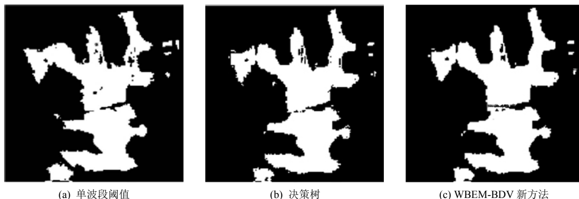
Figure 3. Water body extraction results of Baijia Lake by SPOT-5 remote sensing 图 3. SPOT-5 遥感百家湖水体提取结果
