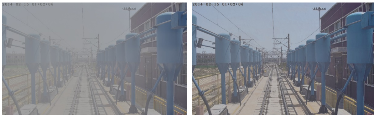
Figure 6. Comparison of rail transit scene image before and after defogging 图 6. 轨交场景图像去雾前后对比
