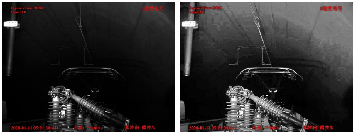
Figure 2. Before and after low light image enhancement for rail scenes
