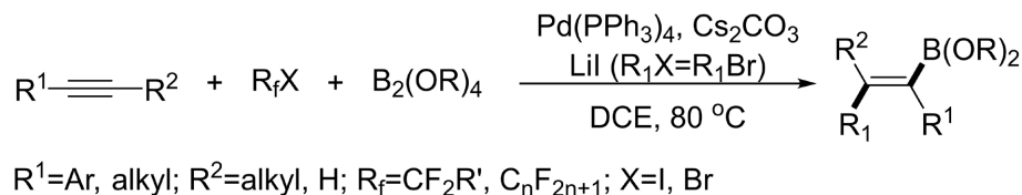
Figure 20. Palladium-catalyzed alkyne fluoroalkyl boration 图 20. 钯催化的炔氟烷基硼化反应
