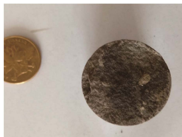
Figure 13. The oil penetrated area on wellbore cores 图 13. 壁心渗油面积
