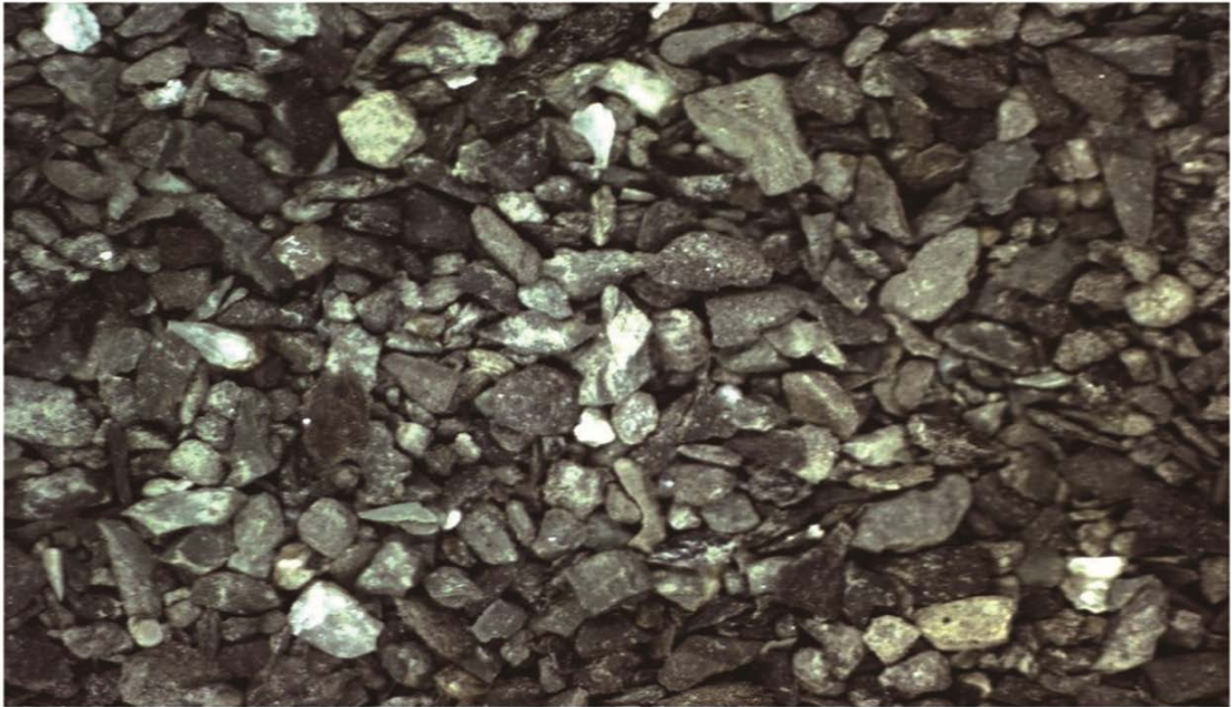
Figure 4. The cuttings at 2950 m of Well SG XX (100 times) 图 4. SG XX 井 2950 m 岩屑(100 倍)
