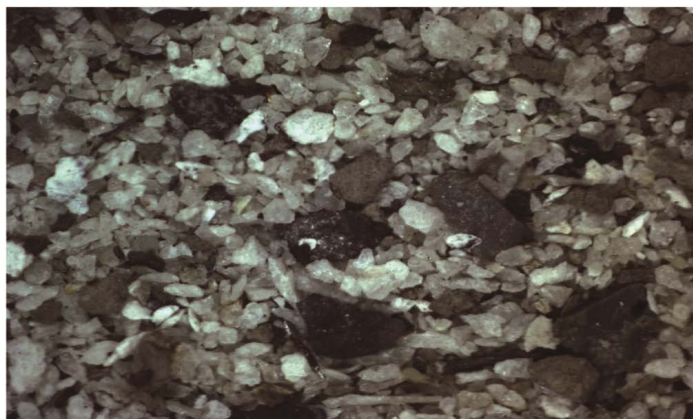
Figure 17. The cuttings at 2994 m of Well DG89 (50 times) 图 17. DG89 井 2994 m 岩屑(50 倍)
