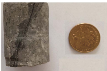
Figure 11. The shape of wellbore coring cracks 图 11. 壁心裂缝形态
