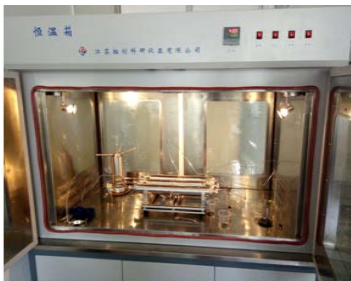
Figure 1. The core physical simulation displacement device 图 1. 岩心物模驱替装置
