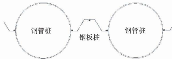
Figure 1. Schematic diagram of standard combination system of tubular piles and sheet piles 图 1. 管板桩标准组合体系示意图
