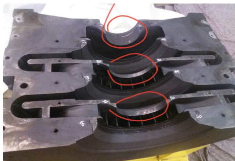
Figure 3. The serious damage of seals in the first, second and third stage shafts 图 3. 一、二、三级轴密封严重磨损
