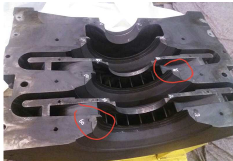
Figure 2. The serious damage of comb seals for second and third stage impeller 图 2. 二、三级叶轮梳齿密封严重损坏
