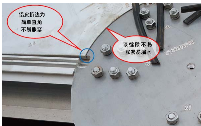
Figure 4. Aluminum sheet folding structure of A Supplier 图 4. A 供应商铝板折边结构
