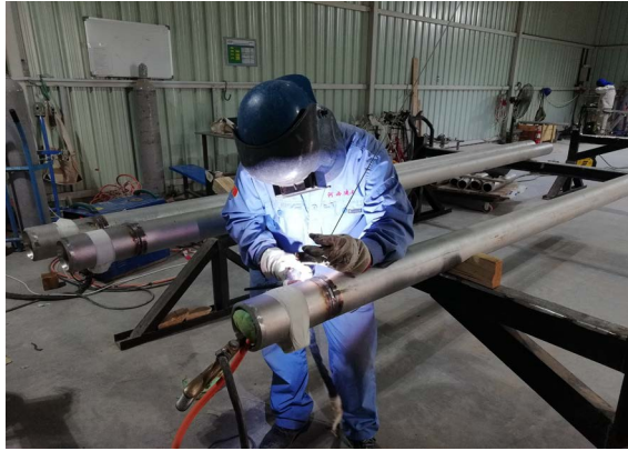
Figure 7. Picture of traditional argon filling method 图 7. 传统充氩方式
