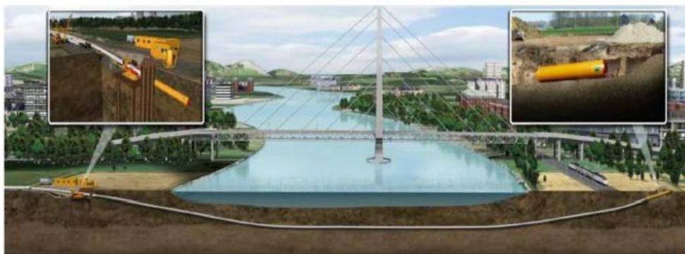
Figure 4. Reference for the direct pipeline crossing profile 图4. 直铺管穿越曲线示意图
