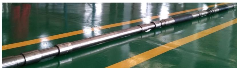
Figure 5. Physical connection diagram of ACP process string placed by syringe in horizontal well
