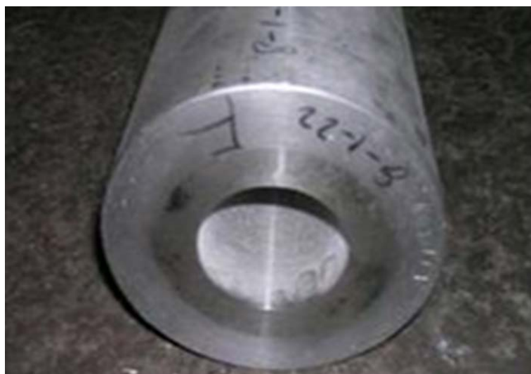
Figure 1. Metallurgical bimetal composite pipe 图 1. 冶金双金属复合管
