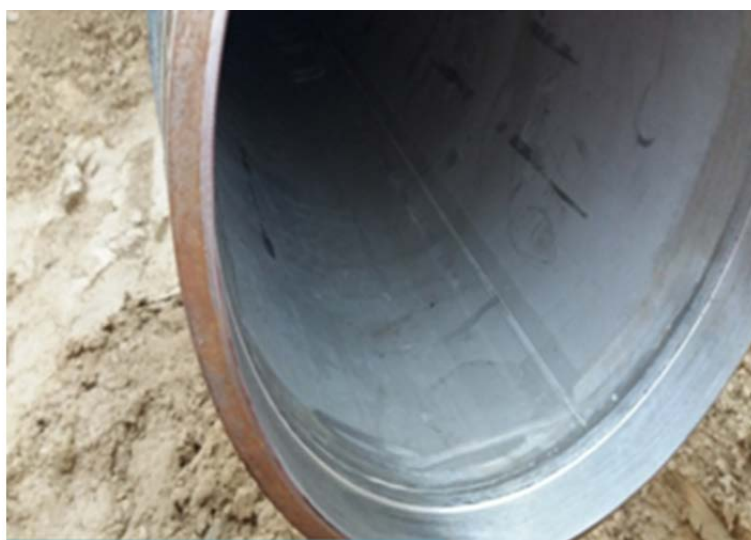
Figure 2. Mechanical bimetal composite pipe 图 2. 机械双金属复合管
