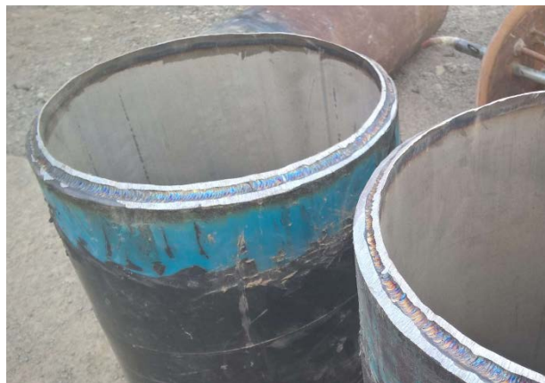
Figure 4. Pipe section surfacing 图 4. 管段堆焊
