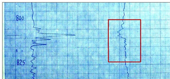
Figure 5. Spontaneous potential curve of foundation well (negative anomaly) 图 5. 基础井自然电位曲线(负异常)
