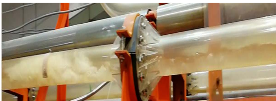
Figure 3. Slug flow pattern appears when the airflow is stable and liquid-carrying at an inclination angle of 10^{\circ} 图 3. 倾角 10^{\circ} 时气流稳定携液出现段塞流流型
