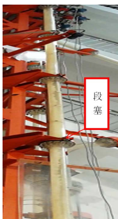
Figure 15. Gas-liquid two-phase flow pattern in the critical state of air-carrying liquid in a 60° inclined well section 图 15. 60° 倾角斜井段气流携液临界状态时气液两相流型
