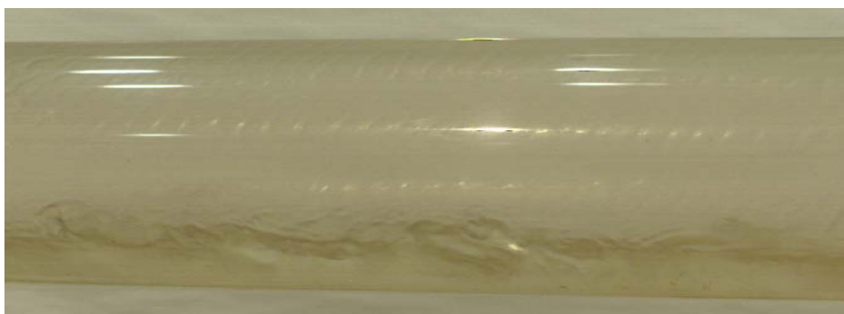
Figure 2. Stable liquid-carrying wave-like flow pattern of air flow at an inclination angle of 15^{\circ} 图 2. 倾角 15^{\circ} 时气流稳定携液波状流流型
