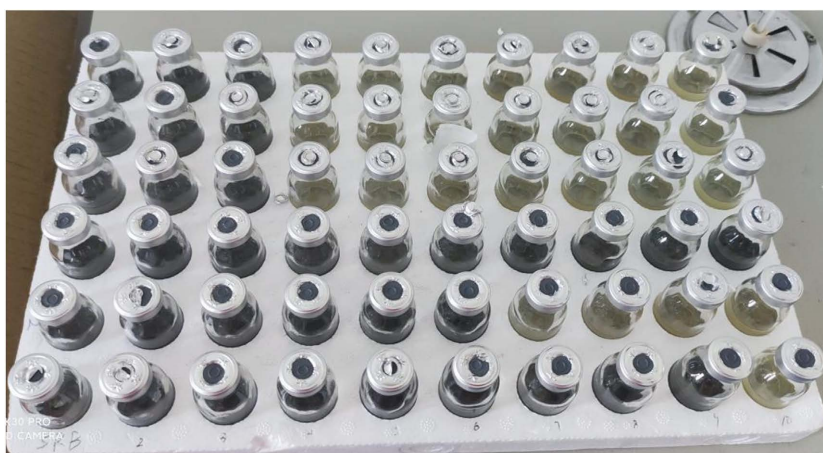
Figure 1. SRB test results (lower three rows)
