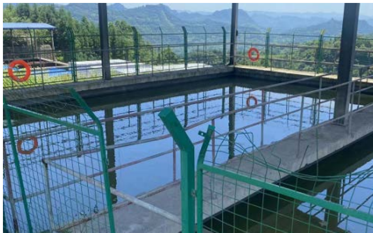
Figure 4. Field photo of water storage test in a shale gas pool after restoration 图 4. 某页岩气水池修复后蓄水试验现场照片
