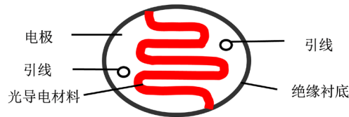
Figure 3. Basic structure schematic diagram of photo resistance
