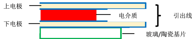
Figure 2. Basic structure schematic diagram of humidity sensitive capacitance
