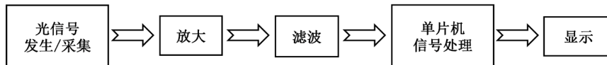
Figure 4. The pulse signal processing circuit design block diagram 图 4. 信号处理电路设计框图
