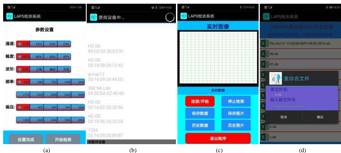
Figure 3. LAPS detection system APP interface. (a) Parameter setting interface; (b) Communication connection interface; (c) Real-time data interface; (d) File operation interface
