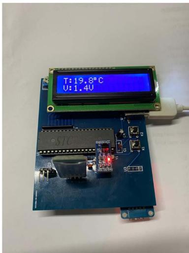
**Figure 5.** Temperature result display
