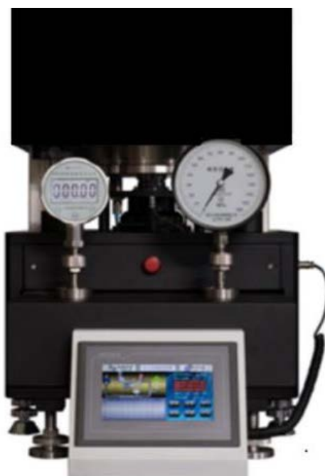
Figure 12. Full automatic gas piston pressure gauge physical diagram
