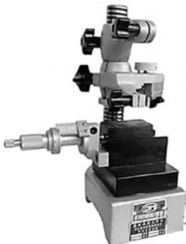
Figure 3. The eddy current sensor calibration bench 图 3. 电涡流传感器标定台架
