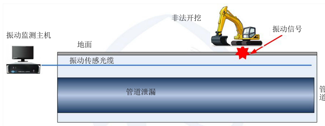
Figure 3. Schematic diagram of pipeline monitoring system
