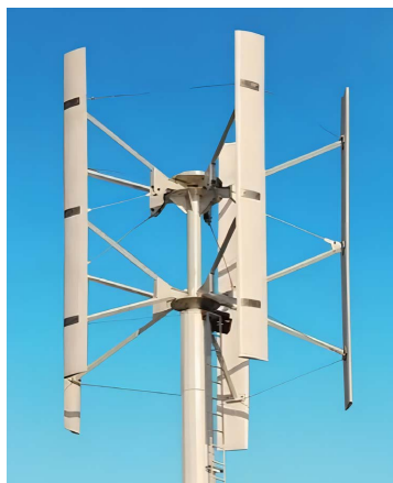
Figure 3. Vertical axis wind power plant 图 3. 垂直轴风力发电装置
