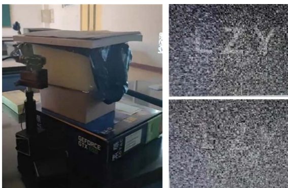
Figure 5. The ghost imaging experimental results by placing smoke as obstacles 图 5. 以烟雾为障碍物时的鬼成像实验结果图
