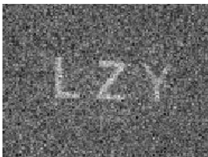
Figure 6. The ghost imaging experimental results by placing rotating ground glass as dynamic obstacles 图 6. 以旋转毛玻璃为动态障碍物时的鬼成像实验结果图
