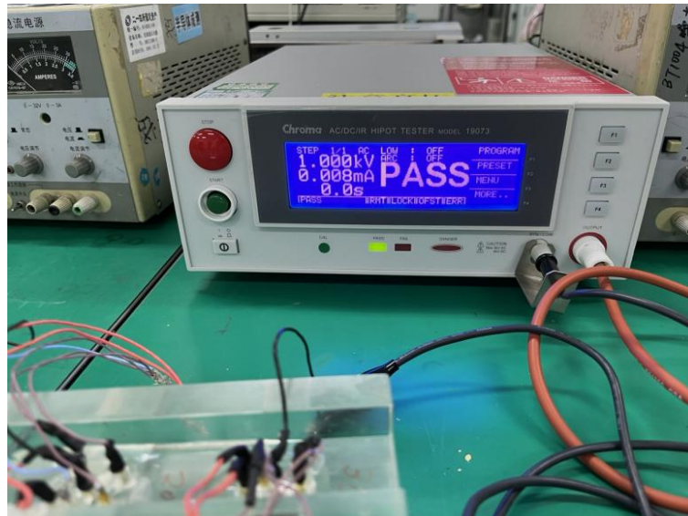
Figure 1. Dielectric voltage resistance test diagram of printed circuit board [3] 图1. 印制电路板介质耐电压实验图[3]
