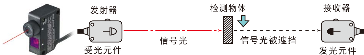
Figure 7. Schematic diagram of laser sensor 图 7. 激光式传感器示意图
