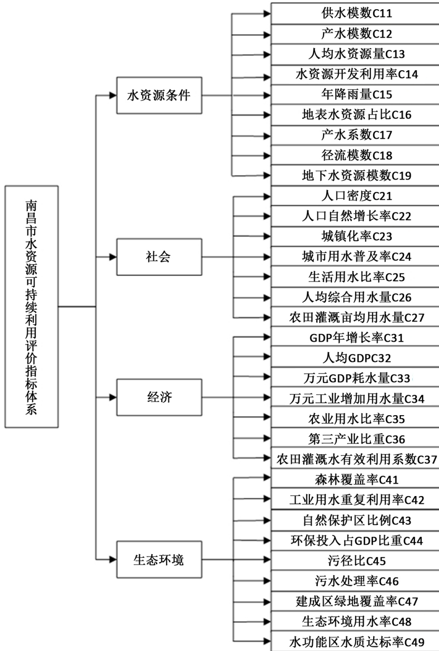
Figure 1. Water resources sustainable utilization evaluation index system of Nanchang city 图1. 南昌市水资源可持续利用评价指标体系
