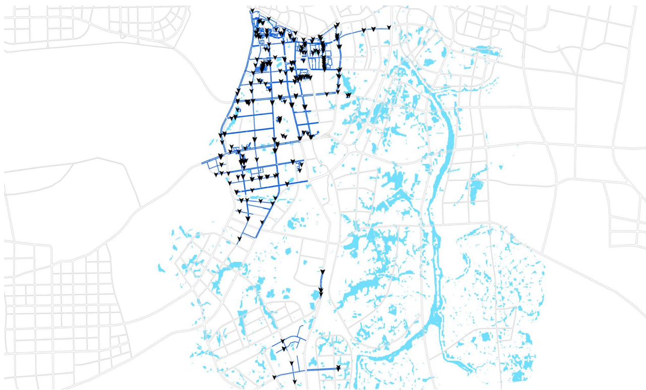
Figure 5. Current hydrodynamic model of rainwater pipe network in Chengnan area 图 5. 城南区城市管网现状水动力模型
