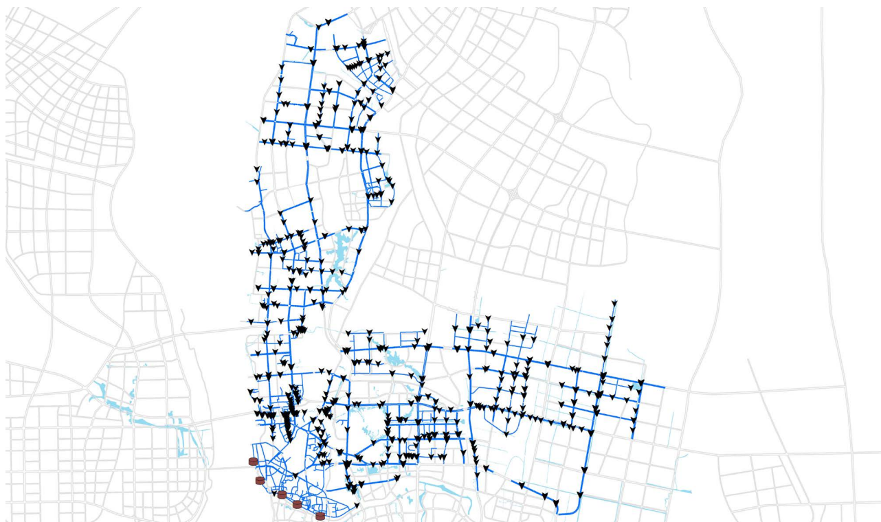
Figure 4. Current hydrodynamic model of rainwater pipe network in Chengbei area 图 4. 城北区城市管网现状水动力模型
