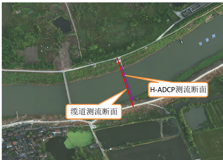
Figure 2. Location of current meter of hydrometric station at Qianhan village 图 2. 前埠村水文站测流断面位置图
