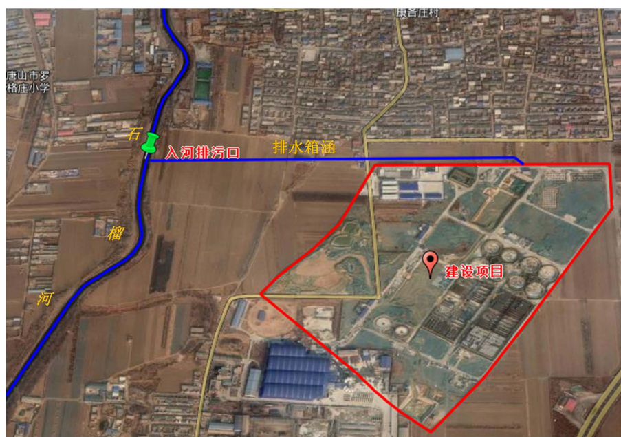
Figure 1. Distribution map of drainage pipelines and river discharge outlets of sewage treatment plants in the northeast suburbs
