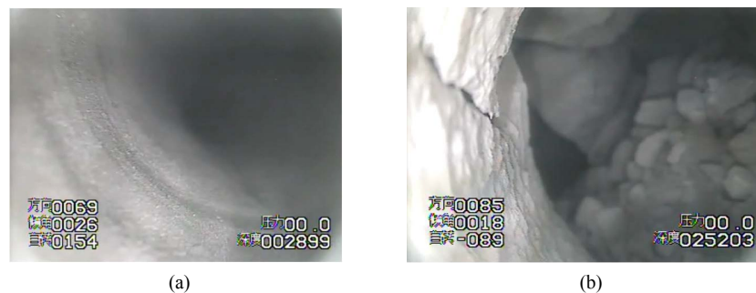
Figure 5. 3# borehole TV camera. (a) 3# borehole was not affected by mining area (2.8 m); (b) 3# drilling area (25.2 m)
