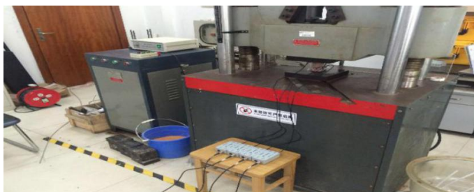
Figure 3. WES-D1000 type electro-hydraulic servo universal testing machine 图 3. WES-D1000 型电液伺服万能试验机
