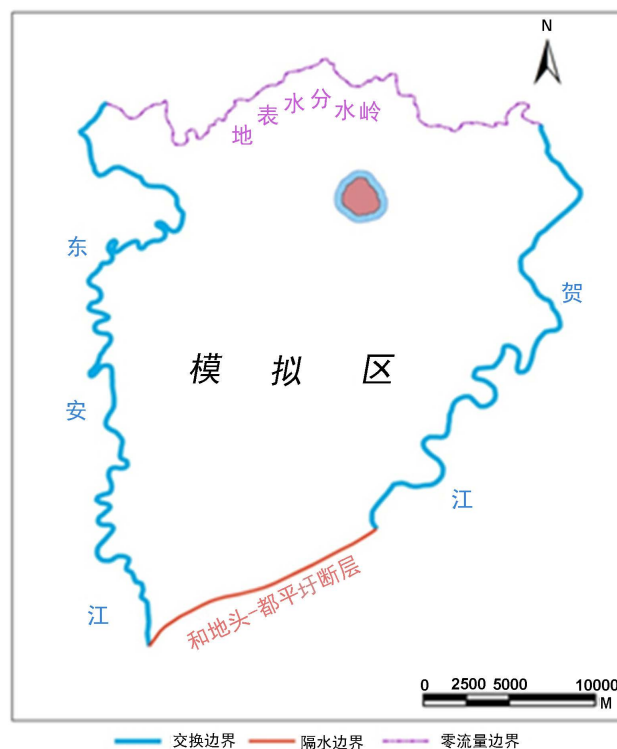
Figure 5. Boundary types of the simulation area 图 5. 模拟区边界条件示意图
