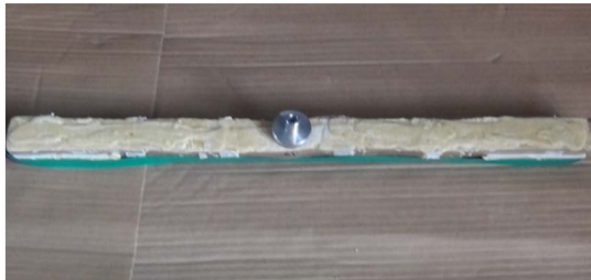
Figure 2. Linear shaped energy cutter 图 2. 线型聚能切割器
