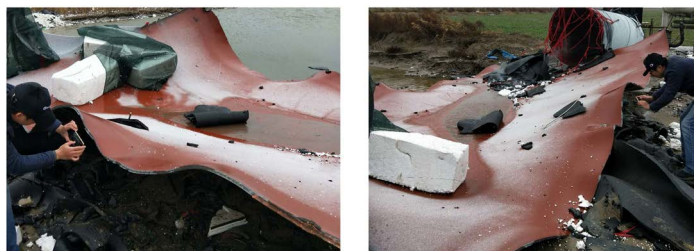
Figure 8. The second test of the overall blasting effect of the steel pipe 图 8. 第二次试验钢管整体爆破效果图
