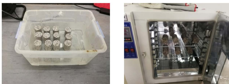
Figure 2. Natural soaking and blast drying of granite
