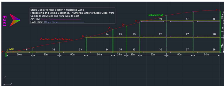
Figure 2. Layout of exploration and mining 图 2. 探采布置图
