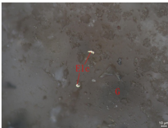
Figure 5. The silver-gold deposits (Elc) are distributed in the gangue minerals (G) in the shape of short veins and granules
