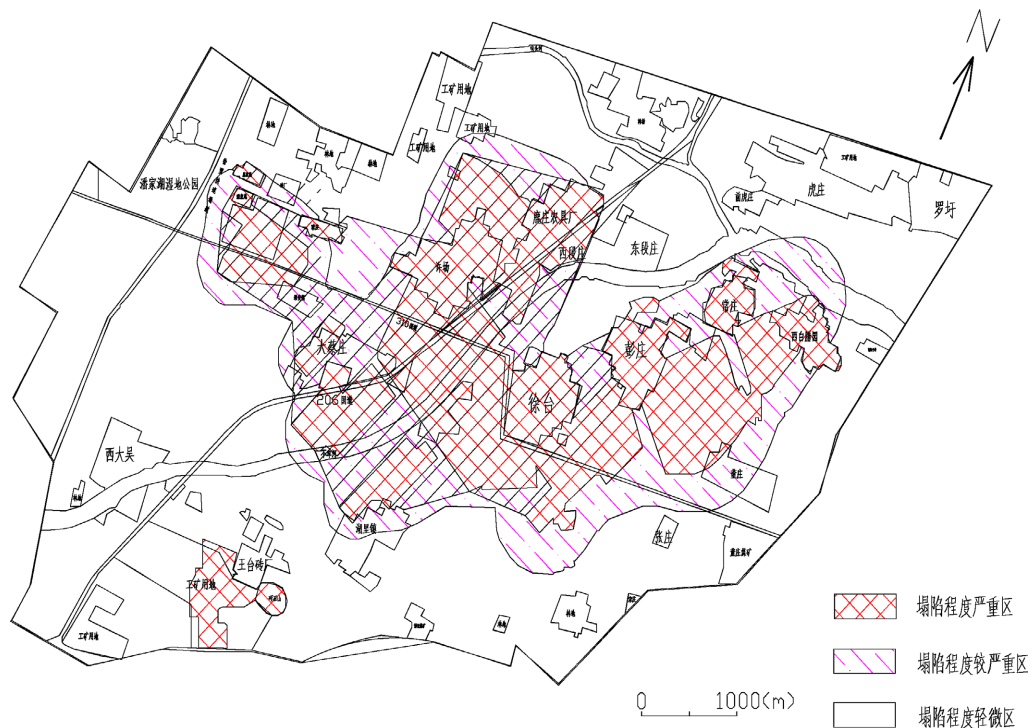
Figure 2. Zoning map of collapse degree in collapse area 图 2. 塌陷区塌陷程度分区图
