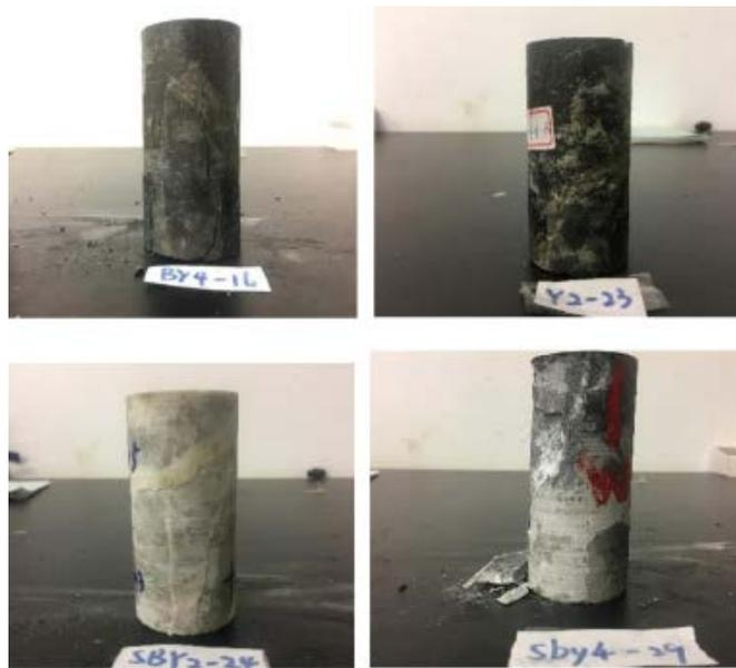
Figure 4. Partially damaged specimens
