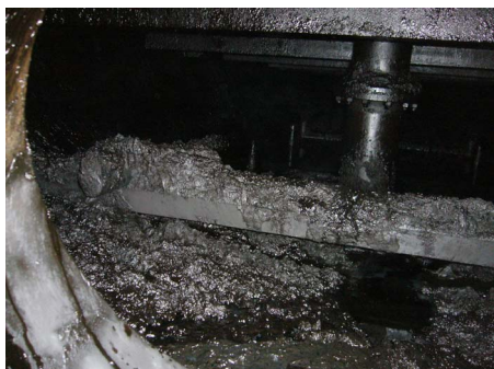
Figure 5. The Two Distillation desalting long time without back-wash tank bottom "silt" serious 图 5. 二蒸馏电脱盐长时间未反冲洗罐底“淤泥”严重
