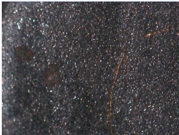
(a) The End surface of Copper electrode
