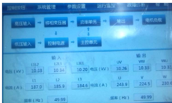
Figure 4. The monitor interface of Soft starter 图 4. 软起动器监控画面
