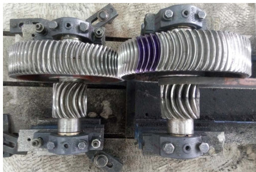
Figure 14. Experimental apparatus to verify the anti-side load characteristics of the involute arc cylindrical
