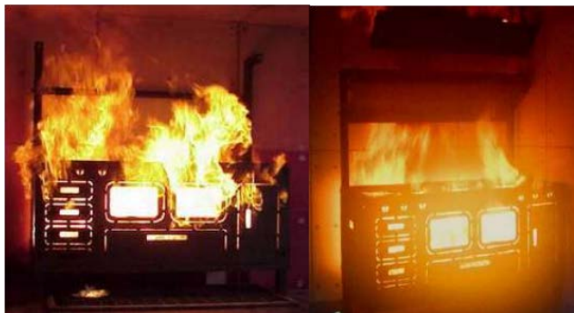
Figure 8. Real map of the kitchen stove burning model 图 8. 厨房灶台燃烧模型实景图
