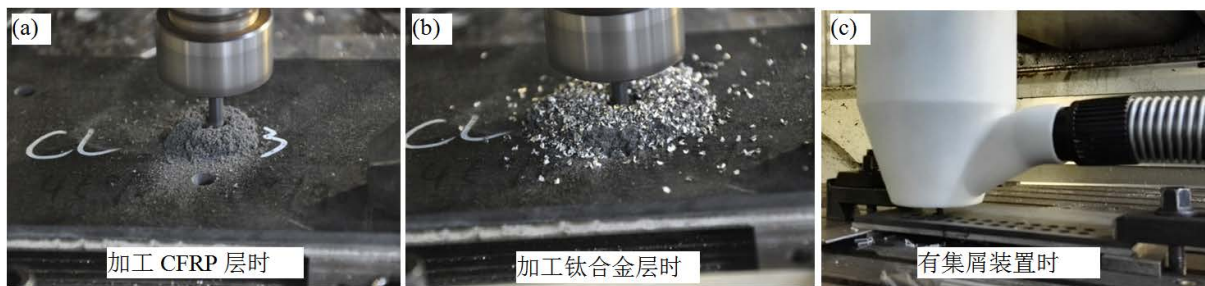
Figure 12. Chips distribution of in helical milling CFRP/Ti stacks, (a) (b) without and (c) with the chip collector 图 12. 自然排屑螺旋铣孔过程中的切屑分布, (a) (b)自然排屑条件下, (c) 有集屑装置时
