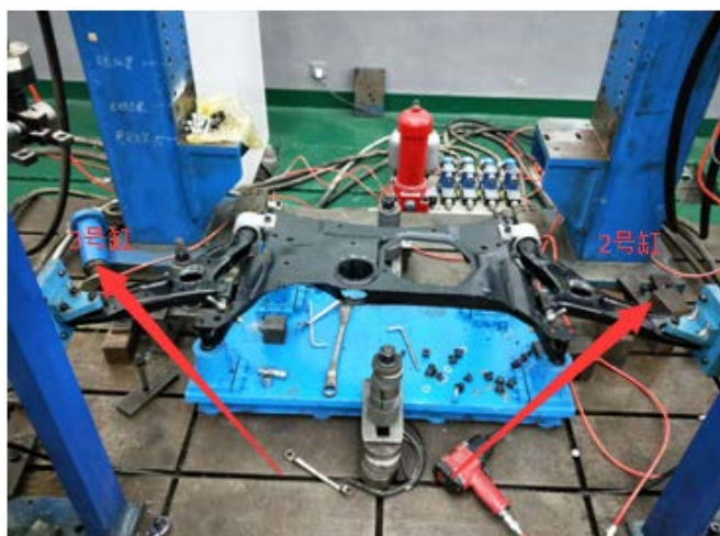
Figure 1. Layout drawing of fatigue test bench for sub frame
